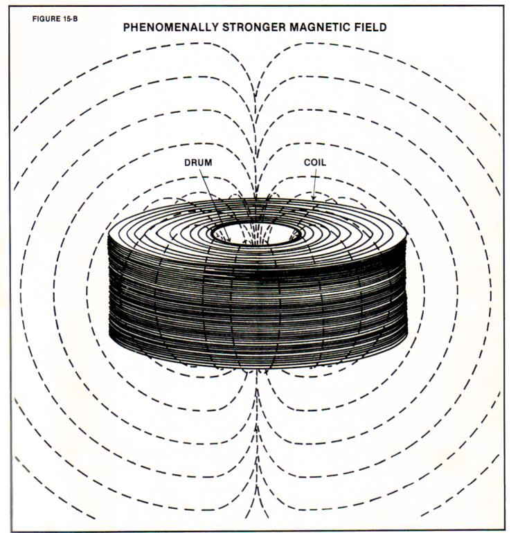
A phenomenally larger current flow would now occur if the current input was stopped and coil 15-B was shorted-out as a result of the collapsing, much greater magnetic field of the 5-gauge wire in coil 15-B. Such shorting would generate an inductance of 25,700 Henries, which is better than <u>8 million times the induc-</u> tance of the 40-gauge coil in Figure 15-A above.
