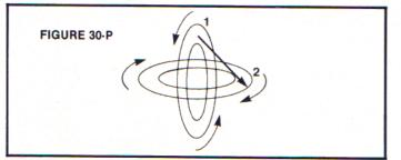
If one pivots the gyroscopic plane of spin from point 1 to point 2, one will observe a noticeable resistance. Such resistance could be called an "inertia effect." If one then *stops* the gyroscopic spin and repeats the same motion from point 1 to point 2, then one will notice very little resistance.
