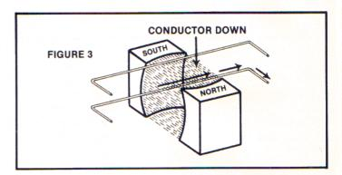
**3.** Flip over the magnet 180° and the direction of the electric current flow will be reversed from that of Figures 1 and 2 above, although the direction and motion of the conductor remain the same (compare Figure 3 to Figure 1 and observe opposite results).
