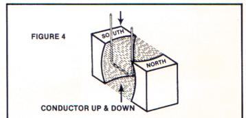
**4.** Push the conductor "down" or "up" in a motion *parallel* to, and through the magnetic lines of force: no electric current will flow despite a vigorous or energetic pushing effort.
