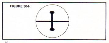
**H.** Consider the following experiment: a two-foot diameter, fiberglass ball has a 10-pound, one-foot diameter gyroscope hidden inside (see Figure 30-H)
