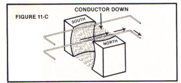
FigureFlip the magnets over 180° and repeat the11-Cactions of Figure 11-A above. The current flow<br/>direction will be *right and opposite to that of*<br/>*Example 11-A even though the force direction is*<br/>*the same.*
