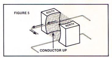
**5.** However, although the conductor can be very slowly pushed at right angles to the magnetic lines of force, the resulting electric current will move at the *speed of light*.
