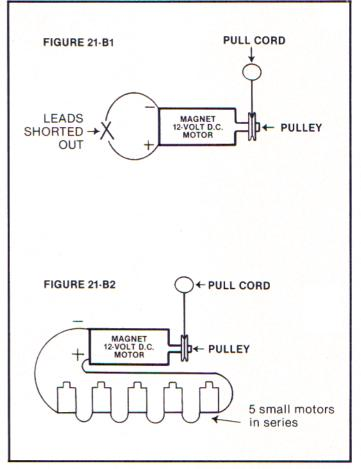
In Figures 21-B1 and 21-B2, the depicted motor also acts as a generator. In 21-B1, if the leads are shorted out with only 1 ohm of resistance in the generator's conductor, *there will be a resistive force equal to the pull-force* that one exerts in pulling the pull-cord attached to the pulley on the motor (generator) shaft. *Reason:* The conductor cuts the magnetic field of the permanent magnets, thereby releasing gyroscopic particles (current) from the magnetic field. *These releas-*
