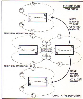
Similarly, with two like poles (see Figure 13-H2) brought together (N to N or S to S) — while they repel each other when placed *bead on*, the models appeared to indicate that the magnets would attract each other when
