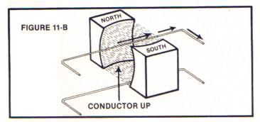
Figure Move the conductor "up" at right angles to the11-B magnetic field and *the current flows right* and opposite to Figure 11-A above.
