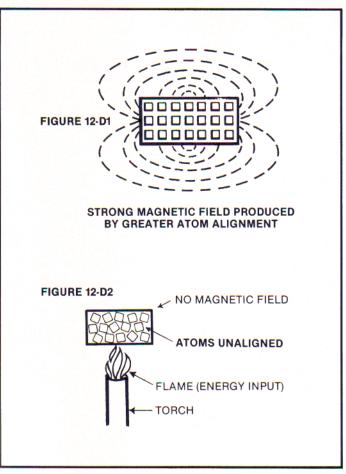
Again, it was obvious to me that the magnetic field disappeared in Figure 12-D2 because the heat input created a random atomic motion and non-alignment within the material. One can clearly see that in Figure 12-D2 one is transferring energy into the system of the magnetic material, *i.e.*, one is not taking energy from the magnetic material and yet the magnetic field virtually disappears.
