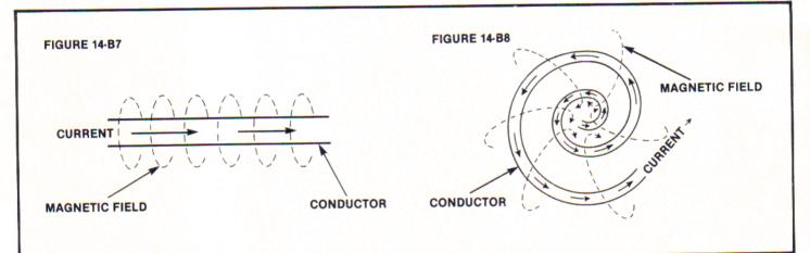
then the current and its associated magnetic field are concentrated, which results in a concentration of the strength of the magnetic field. The student is then provided with the following statement:
