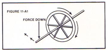
Figure Apply a downward force to the axis of a spin-11-A1 ning gyroscope and it will pivot at a right angle to the force (in this case *pivot left*). Now imagine that this gyroscope has a forward direction at the
