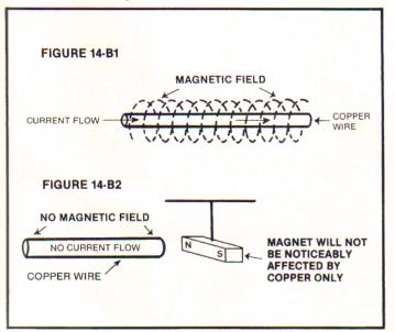
Turn the current on as in Figure 14-B1 and a magnetic field will occur very quickly. Then turn the current off as in Figure 14-B2 and the magnetic field very quickly disappears with no remnant of the magnetic field observed in the copper material. If one then places a magnet close to the copper, it is not observed to be noticeably magnetic. Therefore, one is easily deceived since conventional, *so-called* magnetic materials generate a different result. *Example:*
