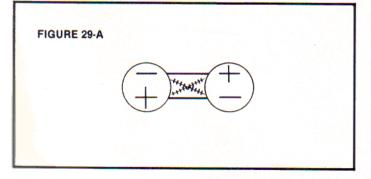
In Figure 29-A, the positive charge within each mass attracts the negative charge and repels the positive charge of the other mass. In addition, the negative charge attracts the positive charge and repels the negative charge of the other mass.
