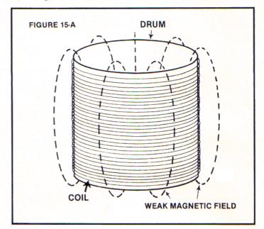
If 100 volts is connected to coil 15-A, then a current flow of approximately 95MA would occur with total power input of 9.5 watts and a resulting weak, magnetic field of .012 Gauss or a mere .000014 Joules of energy stored in this weak, magnetic field.
