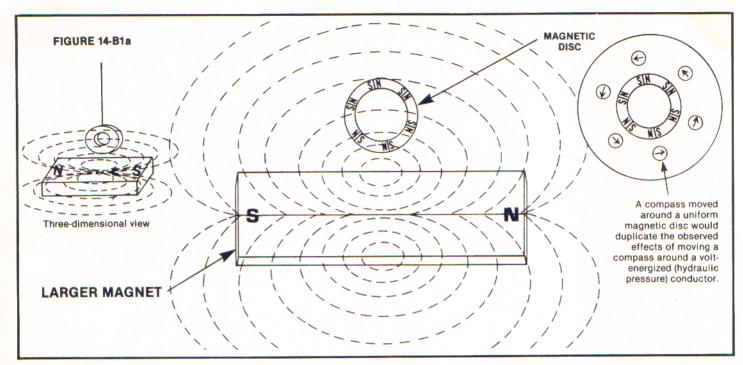
This fact clearly explains why a magnet aligns at right angles to a current-carrying conductor and why a conductor aligns at right angles to a magnetic field.
