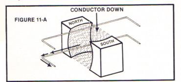
**Figure** Move a conductor down at a right angle to a **11-A** magnetic field and *the current flow moves left*.
