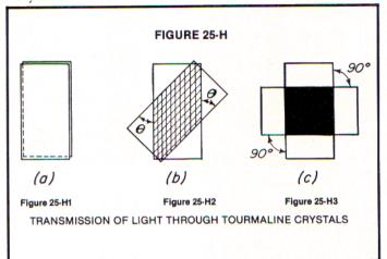
**Figure** Light is transmitted through crystal slabs having **25-H1** their crystalline axes oriented parallel with respect to one another.
