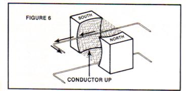
**6.** The conductor can be disconnected from the ammeter, flipped over 180°, reconnected to the ammeter to repeat the same motions of the conductor through, and at right angles to the magnetic lines of force (as in Figures 1-3). Identical results of the electric current flow will then be observed even though the conductor has been flipped over 180°. (See Figures 5 and 6: the conductor in Figure 6 has been flipped over 180° from that of Figure 5, yet the direction of current flow is identical.)
