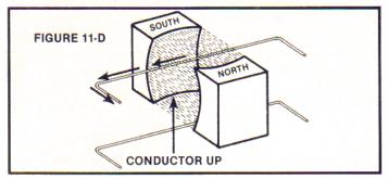
**Figure** Repeat the actions of Figure 11-B and *the current* **11-D** *flow will be left and opposite to Figure 11-B even though the force direction is the same.*
