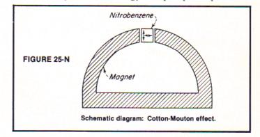
**O.** All of the above processes — which involve producing double refraction in a normally isotropic medium via the application of mechanical deforming forces, magnetic fields, and electrical fields — have a basic similarity: in each case, *physical (mechanical) strains* are produced within the medium which accordingly becomes anisotropic.
