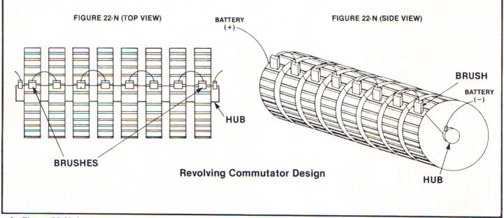
In Figure 22-N the commutator and brushes can simply be multipled two or three times over the original commutator as depicted in the commutator photographs on page 64. The commutator pictured in Figure 22-N has eight breaks and fires simultaneously such that the GAP distance the spark has to travel is multiplied by a factor of eight. Such a mechanical configuration multiplies the
