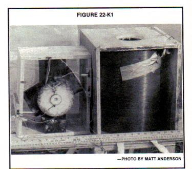
In prototype 22-K1, the FIRING SEGMENT on the commutator switch is 3/8'' wide, the SHORTOUT SEGMENT is 1/8'' wide, and the GAP between the FIR-ING and SHORTOUT SEGMENTS is 1/16'' wide. In the configuration of this commutator, the position of the BLANK SEGMENT is combined with that of the SHORTOUT SEGMENT. This is accomplished by simply placing Scotch tape over the SHORTOUT SEGMENT. (See Figure 22-K2.)
