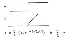
From an oscillograph photo with no load on the system, the coil current rises 0.5 amps in 0.1 sec. when 200 volts are switched across the coil. Thus:
