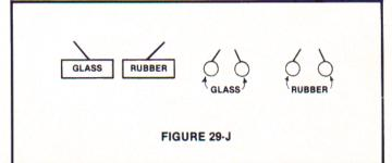
In observing Figure 29-J, it has been said that: "Rubber rods and glass rods can be made to have an electric charge by rubbing the rubber with fur or flannel and the glass with silk. Two electrified pieces of hard rubber rods will be found to repel each other as will two electrified glass rods; but an electrified hard rubber rod will attract to an electrified glass rod."
