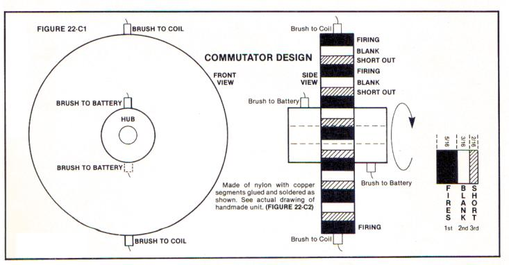
Commutator has 20 Current Input or Firing Positions 5/16" wide, 20 Blank Spots 3/16" wide, and 20 Short Out Positions 2/16" wide.
