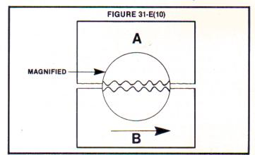
If material B is moved in the direction of the arrow, the the rough surface edges of materials A and B are compressed in *opposite* directions! The rough edges of material A will tend to be ground forward in the direction of the arrow and the rough edges of material B will tend to be ground backward, or in the *opposite* direction of the arrow.
