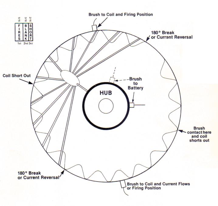
Opposite side of Commutator is connected with Firing Wires to the Hub on the opposite side of the 180° Break. No Short Out Wire is needed on the reverse side.
