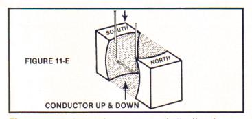
Figure Move the conductor vigorously "up" and 11-E "down" through the magnetic field, *maintain ing the conductor force parallel to the magnetic lines of force and no current flow will result.*
