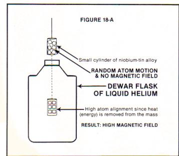
posite to the Curie temperature effect of heat input (energy) into a permanent magnet resulting in atom unalignment, *i.e.*, increased random atom motion, and virtual disappearance of the magnet's field. (See Figure 12-D2 on page 9 for comparison.)
