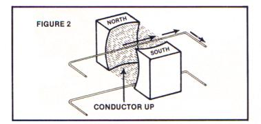
**2.** Push a conductor up and through a magnetic field at right angles to the lines of force and the electric current flows to the right as drawn (opposite to Figure 1 above).
