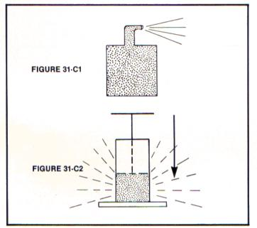
Some scientific books presently teach that a compressed gas cools or loses heat when it expands (see Figure 31-C1), and that a gas gains heat when compressed (see Figure 31-C2).
