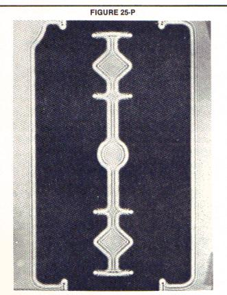
Fresnel diffraction effects in the shadow of a razor blade.
