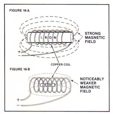
If 1 amp of current goes into Figure **16-A**, a noticeably larger magnetic field occurs than in Figure **16-B** (for the same current input).
