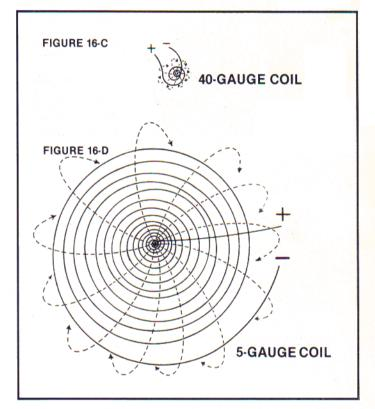
If 1 amp of current goes into Figure **16-C**, a noticeably smaller and weaker magnetic field occurs than in Figure **16-D**.
