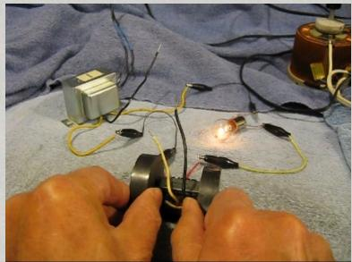
Instead of using magnets, a DC voltage applied to another winding can also cause the core to saturate. This is the basis of a magnetic amplifier circuit.
