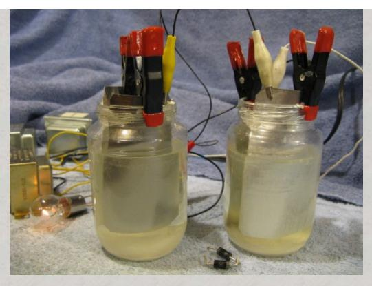
These borax rectifiers are crude as compared to modern silicon diodes but I was still able to observe an amazing power gain of around 450 while using them in the mag amp circuit.
