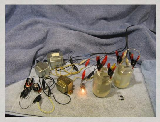
I was curious to see if homemade borax rectifiers (in the two jars) could be used instead of modern silicon rectifiers to increase the gain of the mag amp circuit. The answer is: They can indeed.
