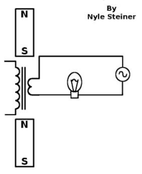
The lamp glows brighter when the magnets are near the transformer. The magnetic field saturates the core, lowering the inductive reactance in series with the lamp.
