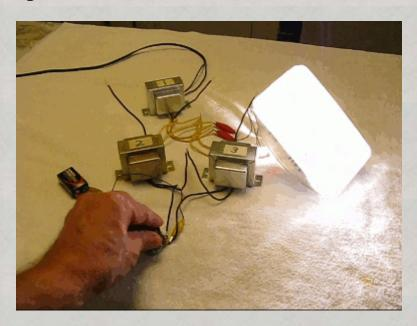
A magnetic amplifier is a circuit that uses changes in core saturation of an inductor to bring about amplification. A small amount of DC current change from the 9 volt battery and a 1k pot can cause a large amount of AC current change through a car headlight.
