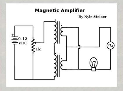
The circle with the sine wave symbol in the center is an AC power supply. In the case of the circuits described here, it is typically a 12v transformer powered from a 120 V 60 HZ outlet.
