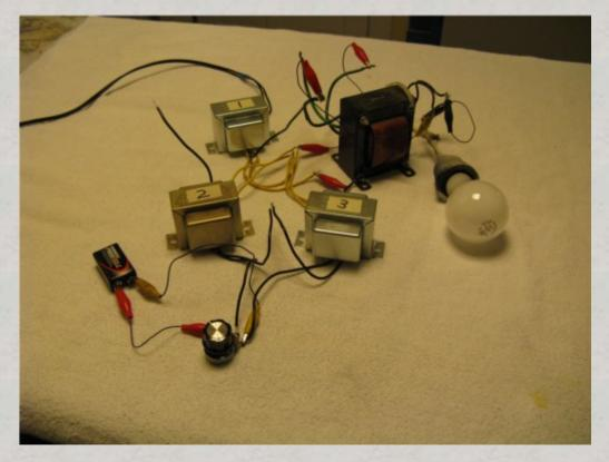
Magnetic amplifiers seem to be best suited for driving low impedance loads in their output. The 12 V car headlight is a typical example. By connecting a step up transformer to the output of one of my 12 V transformer mag amps, I was able to control a 120 V 60 Watt lamp.
