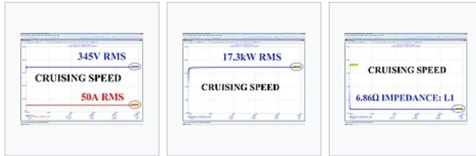
Oscilloscope tracing of the voltage and amperage fed to a motor transformer installed in an electric car traveling at cruising speed simulated in Micro-Cap analog simulator.
