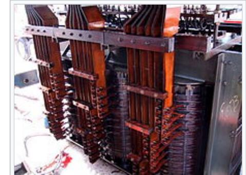
In an [electric arc furnace](#), the transformer has a heavy copper bus for the low voltage winding, which can be rated for tens of thousands of amperes. They are immersed in oil for cooling and insulation, and are designed to survive frequent short circuits.
