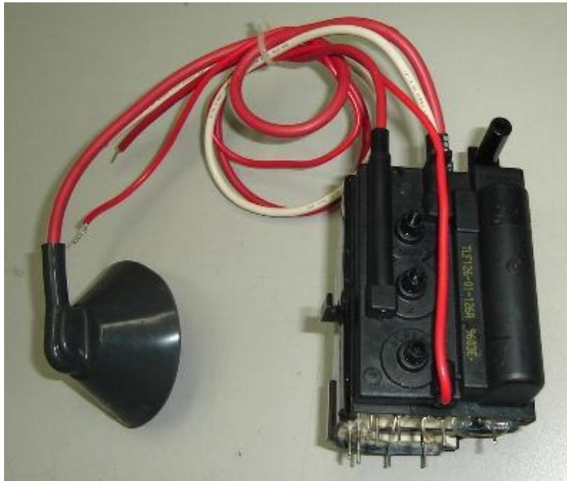
Now for the tricky part, identifying the pins. Set your voltmeter on "beep when shorted" and start testing the pins. Once your voltmeter beeps, check out the resistance. If it's around .6-1, you've found your primary coil. Solder two wires to those terminals and leave them loose for later on. You now need to wrap a feedback coil, which consists of about 6 turns of insulated wire on the outer ferrite core. Once finished, it should look something like this:
