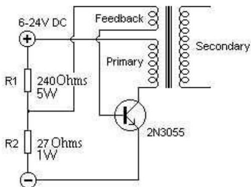
identified the "streamer-output", take the other wire and ground it. It's very rare that the red wire will be the "streamer-output", since that output is (usually) the positive. However, there are many different kinds of flyback transformers, exceptions may occur.
