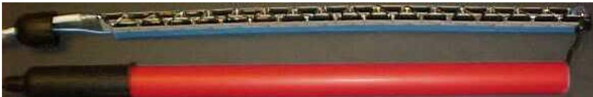
This particular voltage multiplier was slid into the casing of a dead fluorescent light batton for use as a compact source of HT for an ozone generator.
