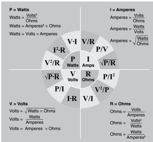
Ohm's Law defines the relationships between (P) power, (V) voltage, (I) current, and (R) resistance. One ohm is the resistance value through which one volt will maintain a current of one ampere.
