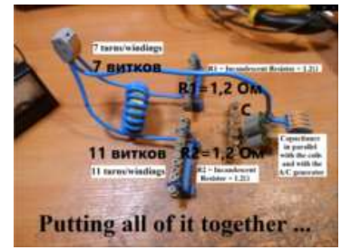
Building the circuit to test a shorted transformer.
