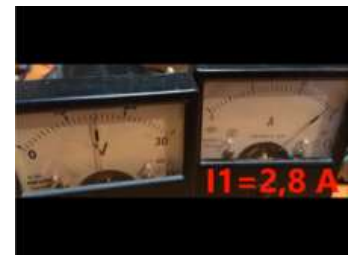
Measuring the total amperage of the circuit: I1.
