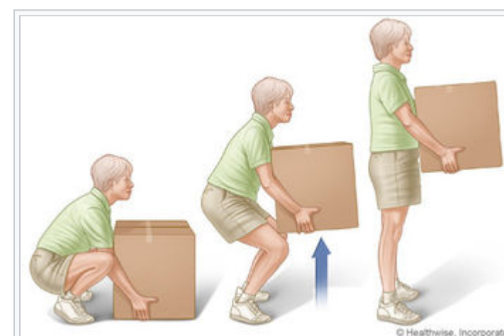
Figure 1: Lifting a box requires a specific amount of energy , no matter how quickly the box is picked up. Lifting faster will change the amount of power but not the amount of energy . [1]
