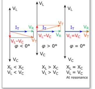
In the series circuit, the same current flows through the resistor, the inductor, and the capacitor, but the individual voltages across the components are different. The phasor diagram shows the  $V_{\mathsf{T}}$  voltage of the ideal sine voltage source. The voltage drop on the resistor  $V_T$  is shown on the horizontal axis in phase with the current that flows through the circuit. The inductance voltage vector  $V_L$  lags the current in the inductance
