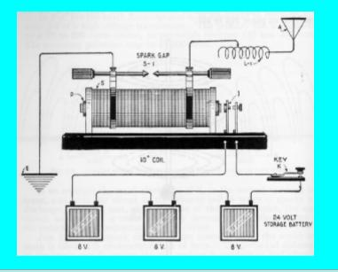
These high currents would charge the antenna, then discharge across the sprak gap electrodes to ground. This action would produce magnetic waves for each discharge across the Spark Gap electrodes. The antenna was connected to the induction coil by means of another coil with a moveable tap. A broad band wave would then be radiated from the antenna.
