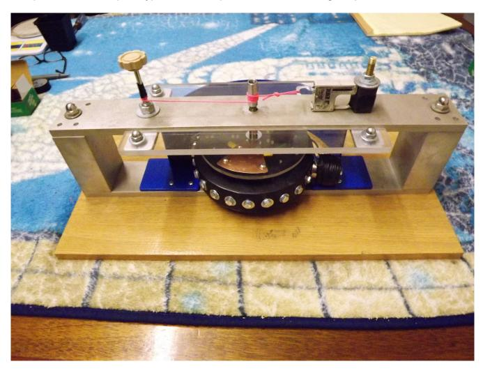
The output is 270 watts running at 611 rpms
