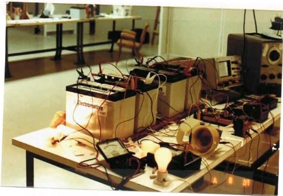
PICTURE 3 Tesla/Brentte/Bedini Switching device loaded with two 110V light bulbs, 110V fan and a 12V 75W quartz lamp.
