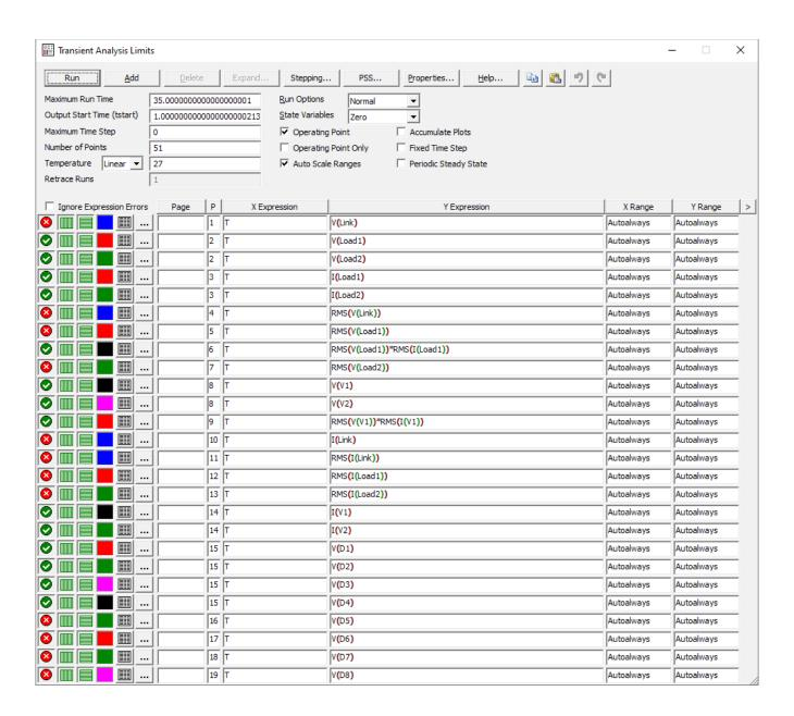
Modified transient analysis settings to zoom into a closeup view of 1 & ½ milliseconds...
