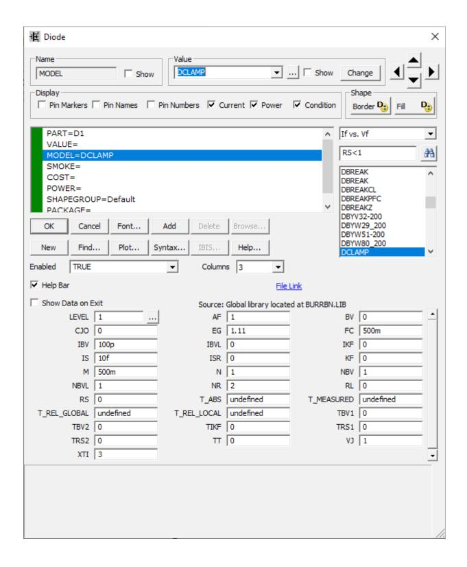
To reduce the chance for "matrix is singular" convergence errors, I add a minute quantity to reactive parameters and series resistances to capacitors and coils and sometimes to spark gaps...
