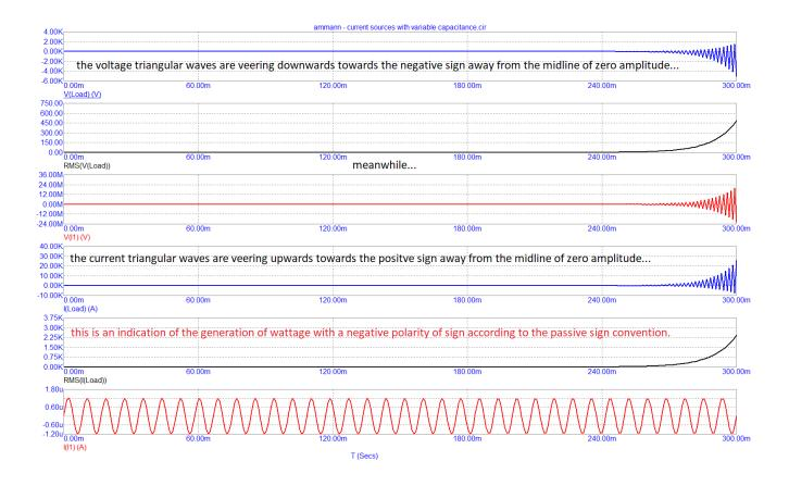
...due to the Load voltage is veering downwards (towards the negative) and the Load amperage is veering upwards towards the positive making this an indication of negative watts and the generation of power according to the passive sign convention<sup>14</sup> which is utilized in all flavors of Berkeley SPICE electronic simulators...
