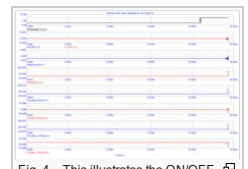
Fig. 4 – This illustrates the ON/OFF state of the neon bulb, in Fig. 2 (above), and the output of four inductive loads. The escalation of wattage is assisted by an inversion of the polarity of current (relative to voltage) resulting from restricting input and preventing any exit of current.
