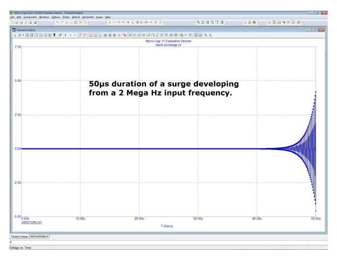
Eventually, the simulation "breaks" due to the inability of the simulator to handle larger durations of analysis when the input frequency is above 1 Mega Hz ...
