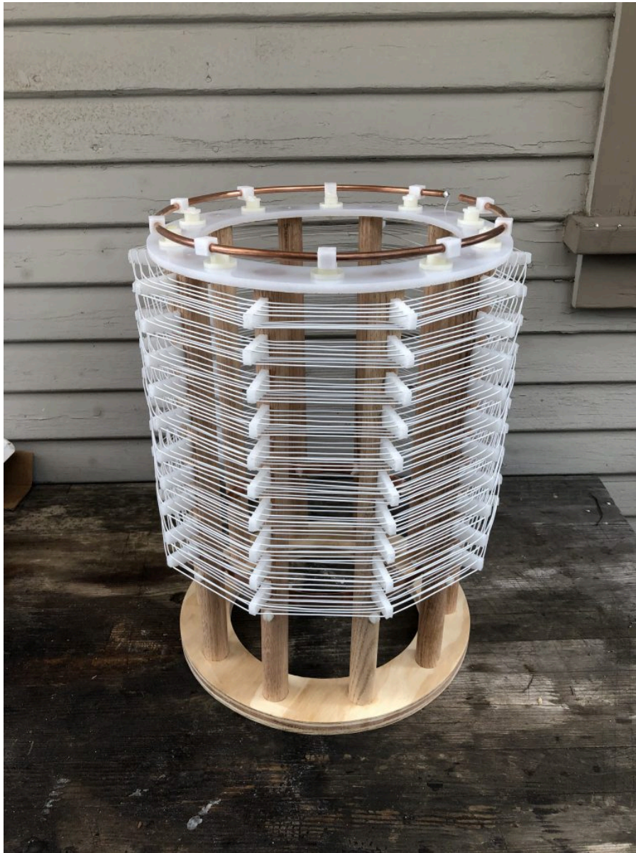
Fig. 4. – Top view of completed coil showing the potential ring affixed to the final windings.
