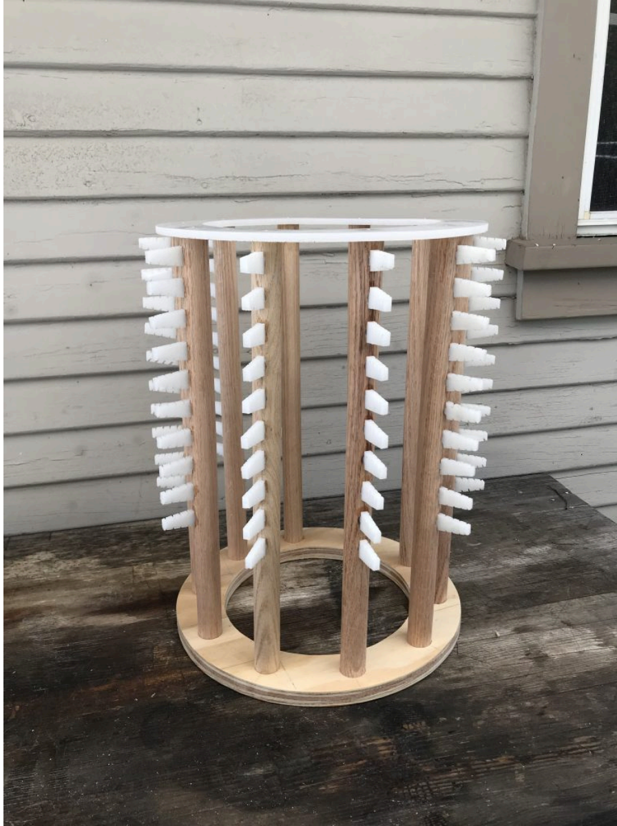
Fig. 2. – Initial construction of the potential coil, displaying the triangular insulator supports of HDPE material.
